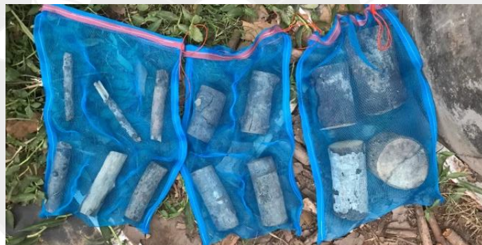
Figure 3.3 Wood Preparation for Wood Degradation Studies
