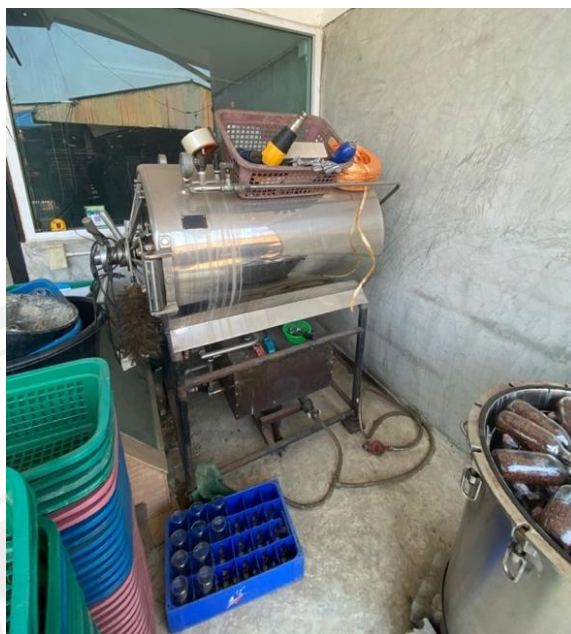
Figure 4.16 Pressing Machine of Materials from Rubber Wood Sawdust for Mushroom Spawn Cultivation Invented by Khun Pairoj for His Own Use
