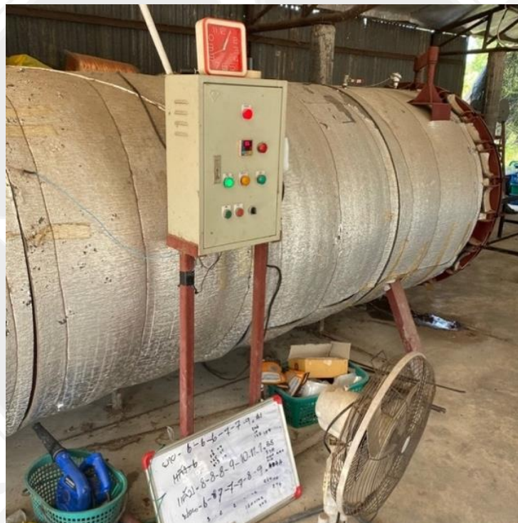
Figure 4.15 Steaming Oven of Mushroom Spawn Invented and Developed by Khun Pairoj to Steam the Raw Material Used of Mushroom Spawn Cultivation for Cleanliness
