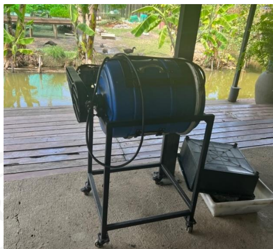
Figure 4.32 Miniature Waste Disposal Equipment Modified by Khun Thaweesak to Process into Compost within 24 Hours by Mixing with Microbes
