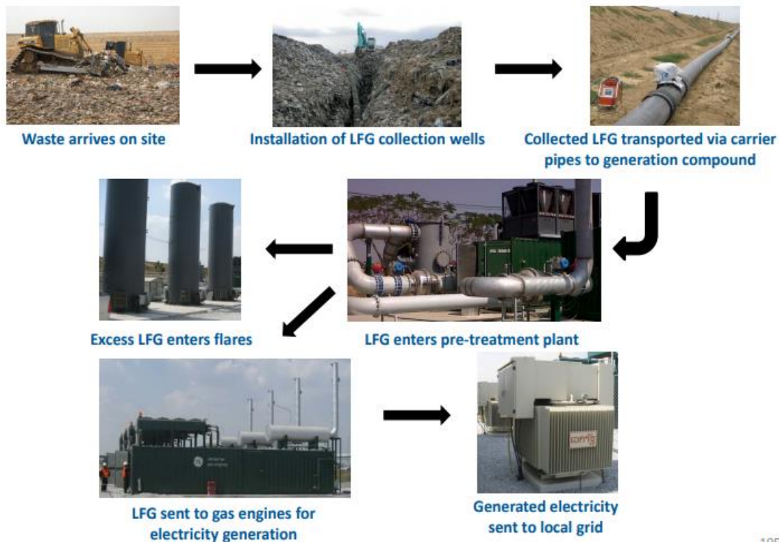
Figure 2.11 Landfill Gas to Energy Process
