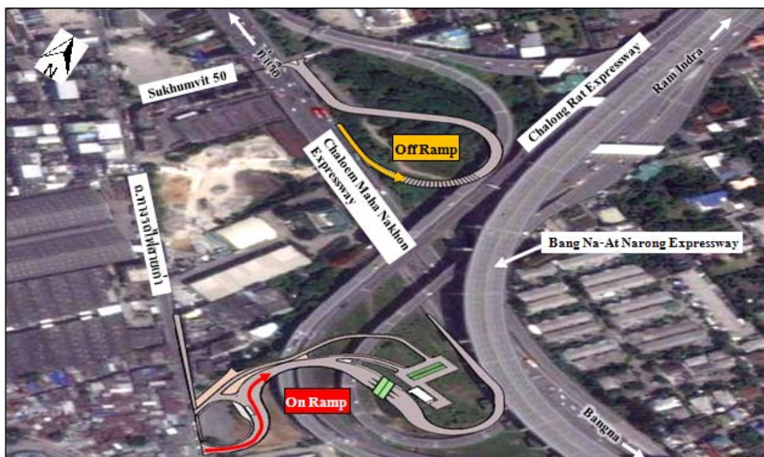
Figure A.5 On-Off Ramps Chaloem Maha Nakhon Expressway Source: Expressway Authority of Thailand, 2010.
